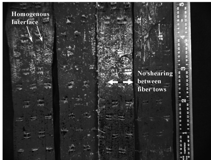
Figure 14. Interfaces obtained in VARTM after in-plane test. Observe a more homogeneous interface, no shearing between fiber tows.
