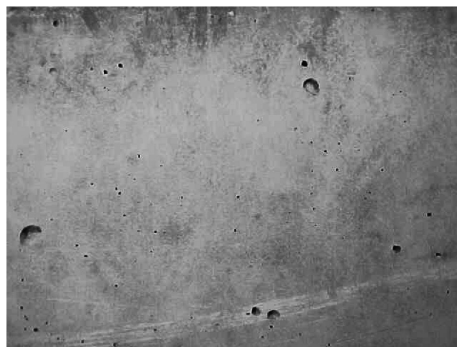
Figure 1. Appearance of average as cast surface 55 MPa concrete.
